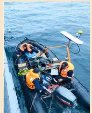
Figura 4: B.A.P. "Zimic" y bote Zodiac MK3 con ecosonda Multihaz 2040-P.
